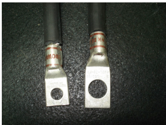
Terminal for 5/16" bolt (left), 1/2" bolt (right)
